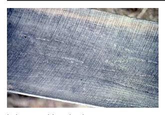
being cut with a circular saw.
